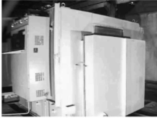
Fig. 6. Setup of controlled water–air cooling of metallic products.
