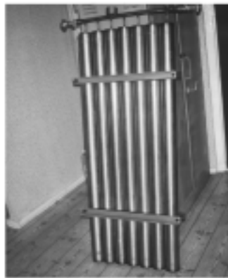
Fig. 4. Balloon for storage and transportation of low-pressure methane in the bound state; it is manufactured from thin-walled steel tubes filled with sorbent.
