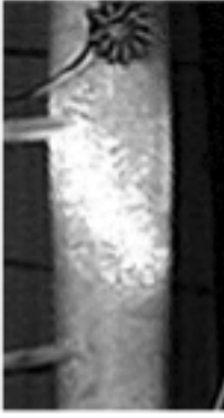
Fig. 8. Inclination instability of the front of filtration combustion of a methane–air mixture.
